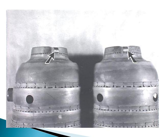
Fractured burner can lugs, as received.
